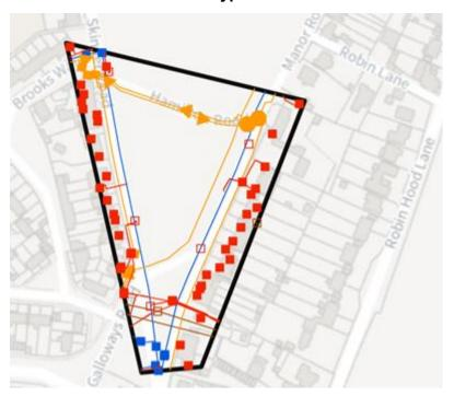
There are SGN pipelines routed through this road (orange) and the electrical equipment is shown in red and belongs to UKPN. There are also water pipelines shown in blue owned by Affinity Water.
