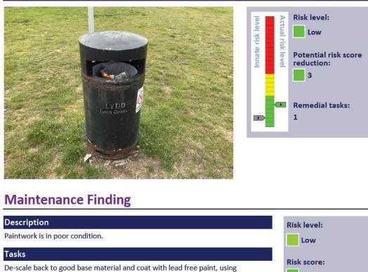
De-scale back to good base material and coat with lead free paint, using appropriate precautions. Repairs may be necessary where corrosion is severe.
