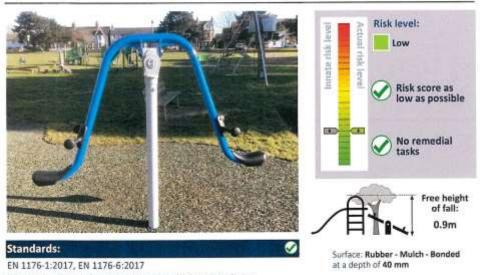
The item and its surfacing (where applicable) meet with the requirements of the relevant standards.
