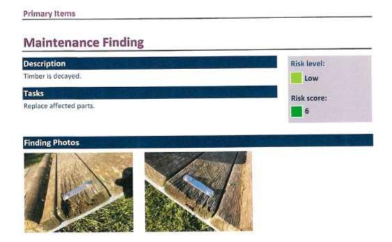
**Primary Items Agility - Stepping Log** Manufactured by (Unknown) Risk level: Innate risk level Low Potential risk score reduction: Remedial tasks: Free height of fall: 0.35m Standards: Surface: Grass EN 1176-1:2017 The item and its surfacing (where applicable) meet with the requirements of the relevant standards. **Maintenance Finding** Description Risk level: Timber is decayed. Low Tasks Risk score: Read the notes for further action. Note Remove and make the ground level. **Finding Photos**
